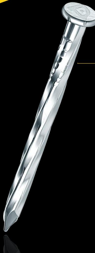
Hinove concrete nails are specially designed fasteners used to secure materials to concrete or masonry surfaces. They are typically made of hardened steel to withstand the hardness of concrete. Concrete nails have a fluted shaft and a sharp, pointed tip that enables them to penetrate the tough surface of concrete without bending or breaking.
